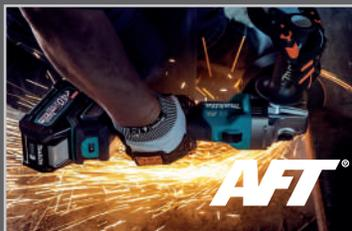
Active Feedback-sensing Technology (AFT®) turns the motor off if rotation of the wheel is suddenly forced to stop.
