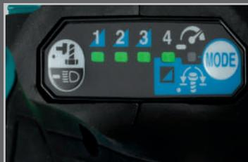
4-speed power selection switch for a wide range of applications.
