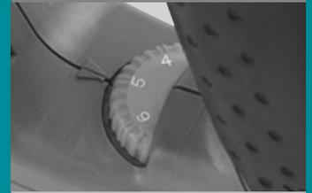
Preset variable speed dial with 6 settings to match the blade speed to the application\*
