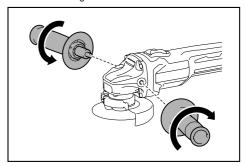
Installing or removing wheel guard (For depressed center wheel, flap disc, flex wheel, wire wheel brush / abrasive cut-off wheel, diamond wheel)
