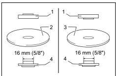
▶ 1. Lock nut 2. Abrasive cut-off wheel (Thinner than 4mm (5/32")) 3. Abrasive cut-off wheel (4mm (5/32") or thicker) 4. Inner flange
