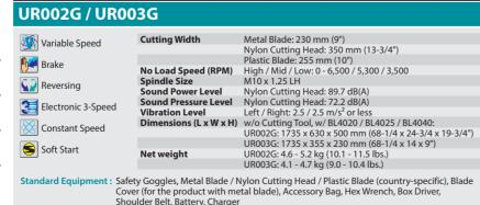
The weight may differ depending on the attachment(s), including the battery cartridge. The lightest and heaviest combination, according to EPTA-Procedure 01/2014, are shown in the table.
