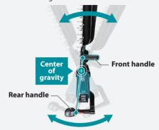
• Due to the inclination of Front handle end, it can be gripped when cutting the top surface, the angle at which the wrist is returned can be reduced, and wrist fatigue is reduced.
