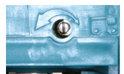
Adjustable automatic chain lubrication
