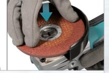
Just one click to attach the accessories easy removal just simply pull the lever
