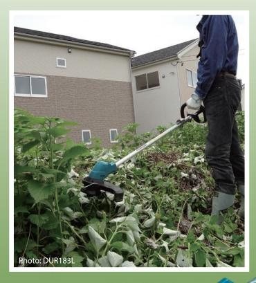
High trimming performance obtained by placing brushless DC motor on the bottom side of the shaft
