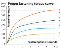
Max mode (4) High strength bolt M16 Hard mode (3) High strength bolt M16
